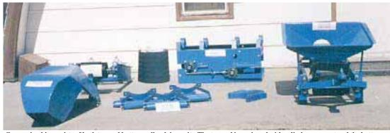
Conversion kit consists of both top and bottom roller drive units. The top end is equipped with a discharge spout and the bottom end is fitted with a 36-in. sq. hopper. There are also belt return rollers and brackets that mount underneath auger tube every 4 ft.
