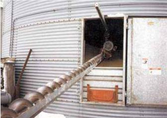
Nuchring attached 18-ft. long section of roller track off a sliding door to top of bin's door frame. He uses the track to roll auger inside the bin.
