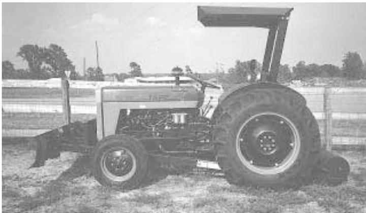
Baird's 6-ft. long front-mount blade is attached to two 12-ft. lengths of steel tubing that run back to tractor 3-pt. Note counterweight on back made from 14-in. dia. pipe.
