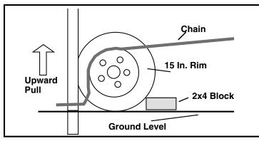
To pull a fence post, Trenary simply wraps the end of a piece of chain around the post and runs it over the top of a 15-in. car wheel rim.
