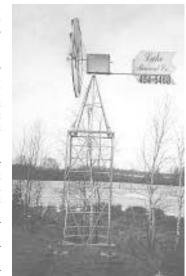
Windmill has a 9-ft. dia. propeller that mounts on a 16-ft. galvanized tower. It pumps air to a pair of "airstones" that create a cloud of fine bubbles.
