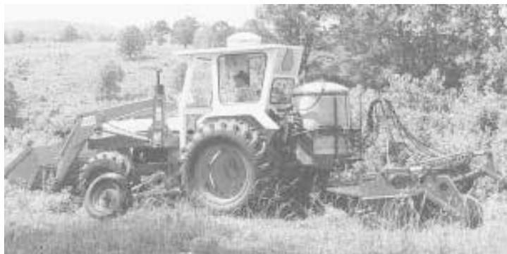
**"Roll-On Applicator" consists of a 10-ft. wide bark scraper followed by an 18-in. dia. herbicide applicator drum.**
