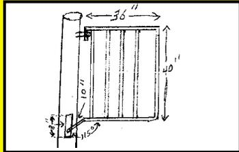
the unhinged end of the gate will rise up and angle out due to the bottom hinge which is offset about 8 inches. When the gate is released, the weight of the gate itself is enough to close it. The heavier the gate material, the harder the slam. Oil companies use 1/2-in. dia. sucker rod for the gate frame and spokes and 1 1/4-in. angle iron for the hinge brackets. **(Dan Shepherd, Rt. 1, Box 111, Lawton, Okla. 73501 ph 580 365-4311)**
