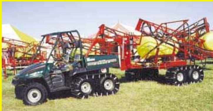
We've been building lightweight "floating" spray rigs for years and introduced our latest new mini-floater at the recent Ohio Farm Science Review. It was hitched to a Polaris "Ranger" 6-WD ATV equipped with a 500 c.c. engine. The Ranger is ideal because it will straddle two 30-in. rows instead of just one with any other 6 or 4-WD ATV we've used before. That leaves an even number of rows on each side of center to follow your planter exactly.
