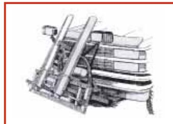
When not in use the forks can be flipped up out of the way against the snowplow frame.
