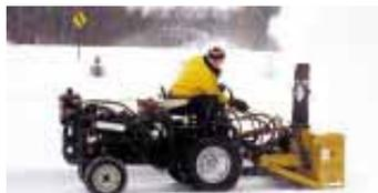
tween the engine and the tractor's original 4-speed transmission. A short driveshaft connects the two transmissions together. He tipped the ring gear over in the differential to run the tractor in reverse.
