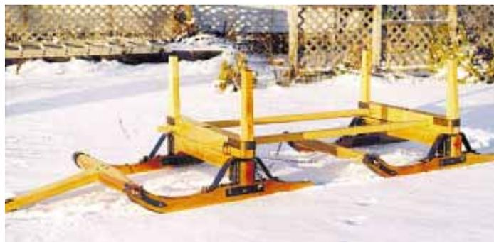
Bobsled's four runner steering system makes it easy to maneuver in tight corners.
