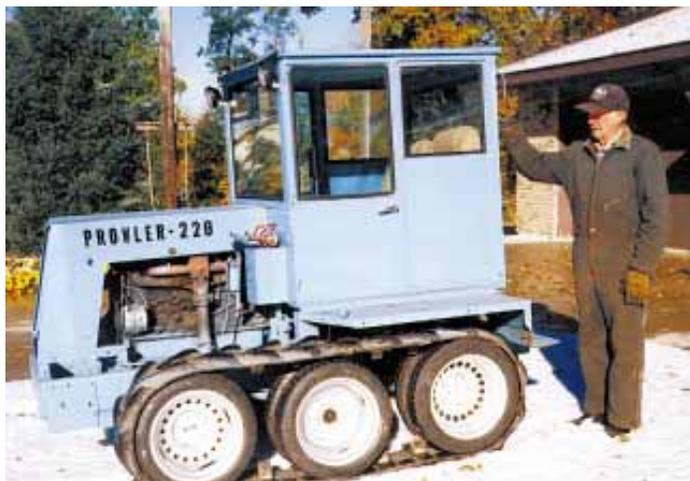
Davis used mostly salvaged parts to build his "Prowler 228". Its 12-in. wide tracks each put 5 ft. of rubber on the ground and are made from two 13 by 6 by 38-in. International M tractor tires with the beads cut off.
