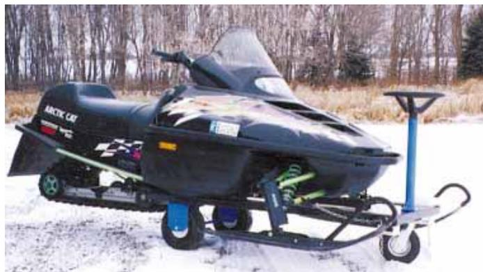
The "SnowVer" is a "pallet fork" that fits under the front end between the skis. It's fitted with two 10-in. dia. wheels that "walk" from front to back of forks to lift sled.
