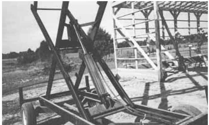
A 5-in. dia., 30-in. long cylinder raises and lowers the lift from a valve on the frame.
