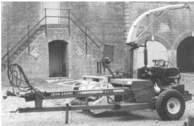
Gay's Deere 3765 forage harvester has 170 hp, thanks to the Leyland 72 hp motor and clutch he mounted behind the machine as a power assist unit.
