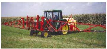
The 60-ft., 3-section boom can be raised up to 4 ft. off the ground. Boom mounts on a quick hitch adaptor that mounts permanently on the tractor frame.
