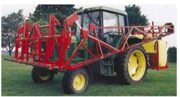
Front-mount boom lets you use the horsepower you've already got to do your spraying and, unlike a pull-type, eliminates wheel tracks that can damage narrow row crops.
