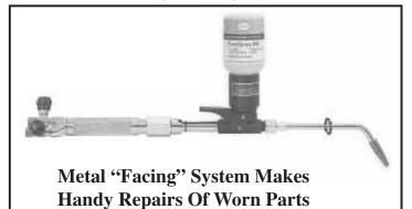
Building up surfaces on worn parts is a lot cheaper than buying new parts in many cases and this flame "facing" system that installs easily on any oxy fuel cutting torch can do the job quickly and easily.
