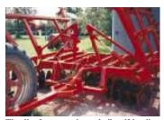
The disc features a home-built self-leveling system controlled by a 4-in. hydraulic cylinder.
