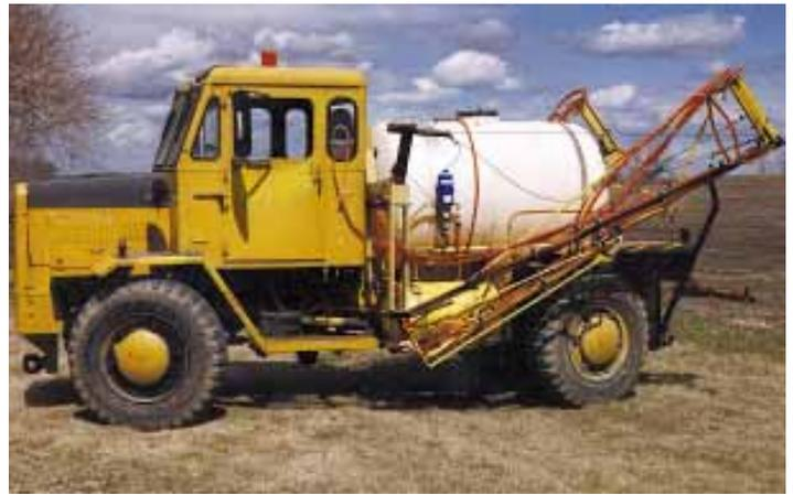
Sprayer features a 6-section, triple-fold boom which is supported by mid-mounted suspension system.
