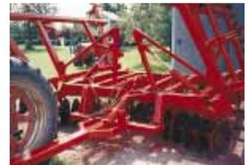
The disc features a home-built self-leveling system controlled by a 4-in. hydraulic cylinder.
