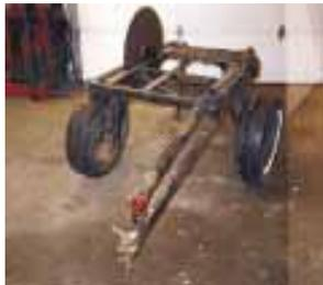
ends of old Ford cars with a 3:1 drive ratio. I ran a driveshaft off the axle end of the differential to the pto and attached the sawblade shaft to the driveshaft. I mounted the mandrels on two-wheel trailers and shielded the blades, of course.
