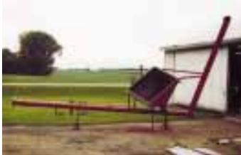
grate, an 8-in. dia. auger, and an 8-in. dia., 11-ft. long "backdraw" auger. The "backdraw" auger allows you to remove grain from a building up to 11 ft. away and dump it into the pit. Prices vary from \$2,000 for a small pit with just a cone and auger up to \$6,000 for a 500 bu. pit equipped with a slide gate and backdraw. Designs are available so you can have your local fabricator build the pit to spec.
