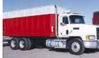
at a 45-degree angle. Elimination of square front corners decreases wind resistance on the road and makes unloading easier. It also
