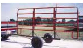
extended the main pipe frame behind the wheels. He then welded and braced two upright pipes with crosspieces to the frame. The crosspieces are angled on the ends so the panels naturally slide to the middle. A couple chain links welded to the posts, with tarp straps attached, hold the panels securely in place. Works great. **(Dennis Shelts, Rt. 1, Box 72, Huntsville, Ill. 62344)**
