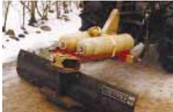
the plumbing lines off the top but kept the threaded end to plug the fiberglass tanks. I filled up the plumbing holes with epoxy resin. I then welded an angle iron rack to lay them on. I welded the rack to the frame of the snow blade. A nylon strap holds the tanks on the rack. The fiberglass weights are weatherproof and can be used on other equipment fitted with the same style of rack. **(Randy Reinke, Orionville, Mich.)**
