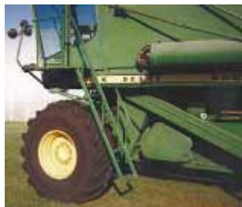
way. I removed the original equipment ladder and platform. The steps and sides are made out of 1 by 2-in. tubing and the railings are 1 by 1-in. tubing. The platform was made out of steel deck plating. The braces between the platform and ladder are made out of 2 by 1/4-in. steel straps.
