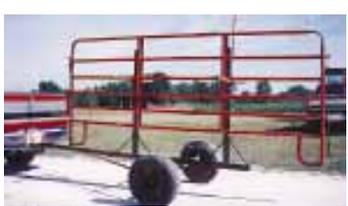
extended the main pipe frame behind the wheels. He then welded and braced two upright pipes with crosspieces to the frame. The crosspieces are angled on the ends so the panels naturally slide to the middle. A couple chain links welded to the posts, with tarp straps attached, hold the panels securely in place. Works great. **(Dennis Shelts, Rt. 1, Box 72, Huntsville, Ill. 62344)**
