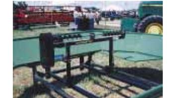
grain out to the edges of the hopper to prevent mounding in the middle of the hopper. It takes the load off the grain tank auger and reduces wear. Can be used with any brand of hopper extension. It's all electronically operated - no hydraulics. Automatically starts and shuts down as needed to keep grain levelled out. It folds down within the hopper for storage. **(Tom Janke, Sales Manager, Cray Co., 237 NW 12th St., P.O. Box 849, West Fargo, N.Dak. 58078 ph 800-247-7335)**
