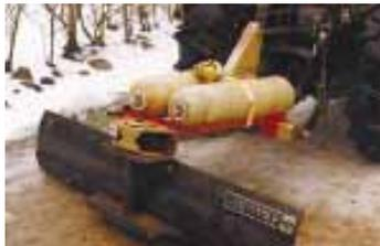
the plumbing lines off the top but kept the threaded end to plug the fiberglass tanks. I filled up the plumbing holes with epoxy resin. I then welded an angle iron rack to lay them on. I welded the rack to the frame of the snow blade. A nylon strap holds the tanks on the rack. The fiberglass weights are weatherproof and can be used on other equipment fitted with the same style of rack. **(Randy Reinke, Ortonville, Mich.)**
