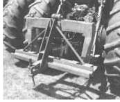
attachment on the 3-pt. hitch. It allows me to level my 24-ft. field cultivator, disc and other implements on the go, which is a time and back saver
