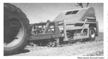
Fisher's tool combines up-front ripping blades with rotary drum that mixes underlying clay with surface sand.
