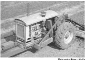
Proto courtesy Farmers weeky Power cart is fitted with a 150 hp Cummins diesel that powers trailing equipment, eliminating need for a larger tractor.
