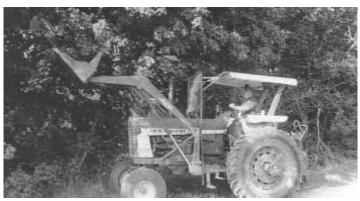
Hydraulic powered brushcutter saws through 3 to 4-in. dia. branches with ease, Brook says.
