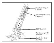
Poly cushions inside gooseneck coupler absorb towing shock.
