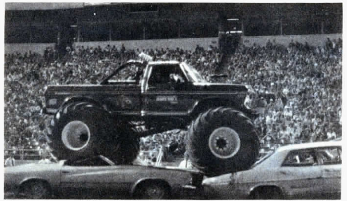
Bigfoot's powered by a highly modified 460 cu. in. Ford engine and has a 5-ton Rockwell axle.
