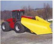
order to reduce wear. We use a Case-IH 7120 tractor that's equipped with an 11-ft. wide, 42-in. high blade to follow behind and clean up. The blade on that tractor can be angled left or right
