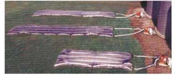
Plastic inflatable solar collector hooks up to the intake side of virtually any existing aeration fan. Air pressure moves air through the solar collector and into the bin.
