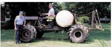
Minick used 3-in. channel iron to build a frame that supports a 300-gal. spray tank behind the seat.
