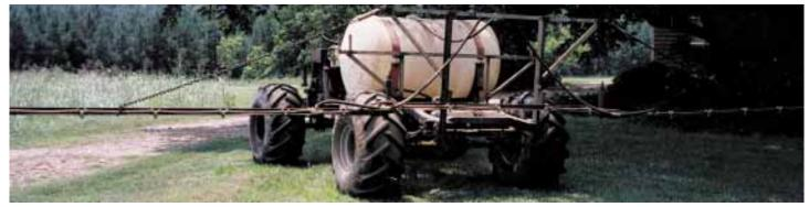
The 4-WD pickup was stripped down as much as possible to save weight and rides on 18.4 by 16 flotation tires, allowing it to float on top of ground without leaving deep tracks.
