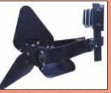
The "Prop" has three blades splayed out at a 45 degree angle from the hub. They dig little water-catching dams as they work through the soil behind ripper. 1 1/4 by 8-in. shanks.
