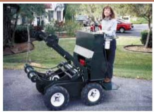
Operator stands on a platform behind a pair of hydraulically-operated clamp arms and a table that tilts forward to pick up a bale.
