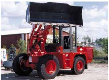
The 4-WD hydrostatic drive rig has a turntable-style loader that rotates 90 degrees to either side for increased maneuverability and easy unloading in tight quarters.
