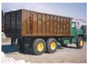
The truck is equipped with a Cummins 6-cyl. diesel engine and automatic transmission and is mounted on 1600 by 24 tires.
