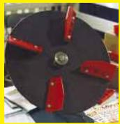
Corrosion-proof plastic blades bolt onto spinner pans and are abrasion and im-
