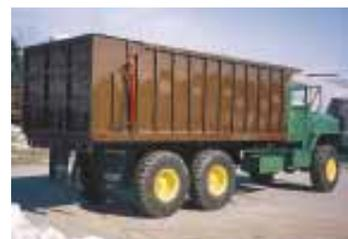
The truck is equipped with a Cummins 6-cyl. diesel engine and automatic transmission and is mounted on 1600 by 24 tires.
