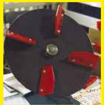
Corrosion-proof plastic blades bolt onto spinner pans and are abrasion and impact-resistant.
