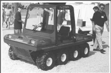
The 8-WD Range Cat 775 ATV is mounted on eight 22-in. high flotation tires and comes with an all-weather canopy and zip-up doors. Tracks are optional.
