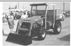
The T-4000 is equipped with a modular 3-pt. hitch and independent live pto that can be used either at front or rear, and a 2,000-lb. capacity hydraulic-operated dump box.
