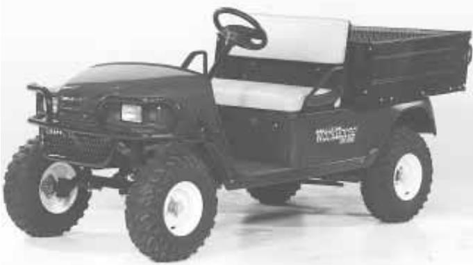
The Workhorse ST-350 mounts on 20-in. high turf saver tires and has an electric-operated dump bed. The two-passenger seat is made from fabric-backed vinyl.
