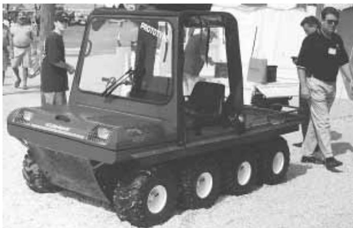
The 8-WD Range Cat 775 ATV is mounted on eight 22-in. high flotation tires and comes with an all-weather canopy and zip-up doors. Tracks are optional.
