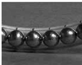
**Rolling motion of the chrome steel balls suspended in a lubricating fluid automatically balances tires.**
