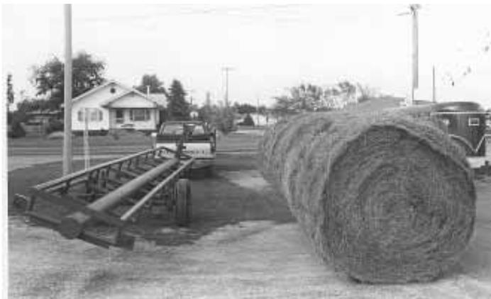
**Bale trailer dumps an entire load simply by flipping a lever on the side. Gravity does the rest.**
