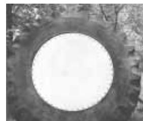
**One side of tire is sealed shut with aluminum sheeting.**
