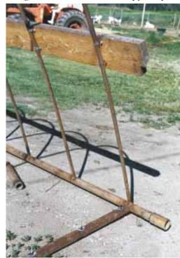
Photo shows how sucker rod fits into base frame. Note sideboard mounted about 4 ft. up the side.
