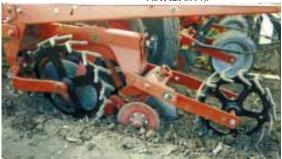
The open wheels don't compact soil like solid wheels, preventing crusting and making it easier to close the seed furrow.
