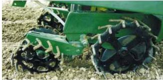
"Posi Close" planting wheels consist of 16-in. dia. steel "baskets" that replace gauge wheels and 12-in. dia. baskets that replace closing wheels.
