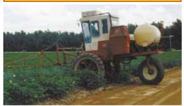
Martin built his sprayer out of an IH 375 swather. It's equipped with a rear-mounted 500-gal, tank and front-mounted 60-ft. boom to cover 16 rows.
