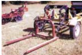
Unit can be fitted with implements such as disks, blades, and hay forks.
