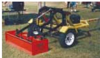
Trailer's 3-pt. hitch is operated by a single hydraulic cylinder that's activated by a remote toggle switch in the cab.
