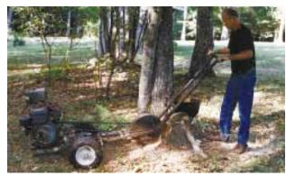
A 16 hp gas engine on front of machine belt-drives a 12-in. dia. flywheel off an old tractor engine. Flywheel is fitted with six cutter blades.
