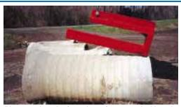
Pipe mover is made of two pieces of square steel tubing - the bottom one is 35 in. long and top one 28 in. long.
