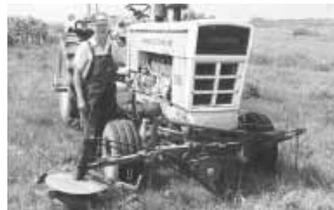
Low-riding mower is belt driven by a shaft running back under the tractor to the pto.
