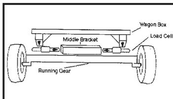
The system consists of four load cells, two in back and two in front. They bolt to a middle bracket that's welded to the running gear.
