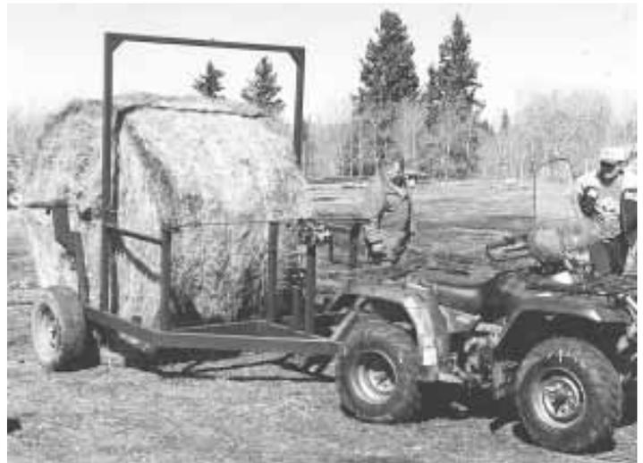
Trailer is operated by hand winches, eliminating batteries and hydraulics.
