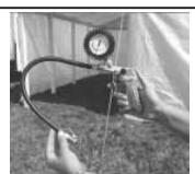
Gun's in-line pressure gauge lets you add, remove air without unhooking.
