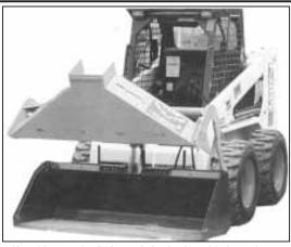
Adjustable spout hooks into existing bucket with three pins.
