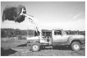
Morrison cut the box off a 1975 Dodge 4-WD pickup and welded a front-end loader onto the frame. He uses loader to spear round bales and load them onto a trailer.
