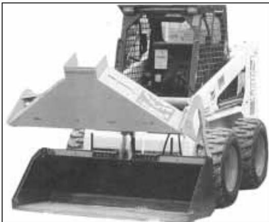
Adjustable spout hooks into existing bucket with three pins.
