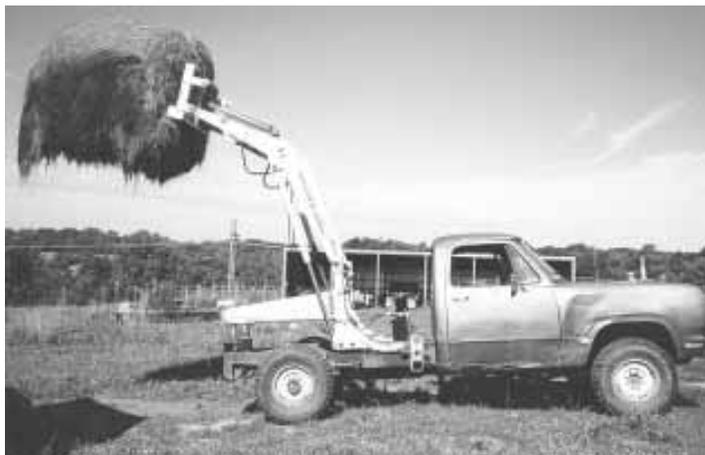
Morrison cut the box off a 1975 Dodge 4-WD pickup and welded a front-end loader onto the frame. He uses loader to spear round bales and load them onto a trailer.
