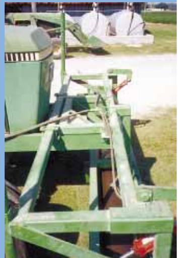
**The 18-in. dia. roller mounts on a steel frame that bolts to sides of tractor.**
