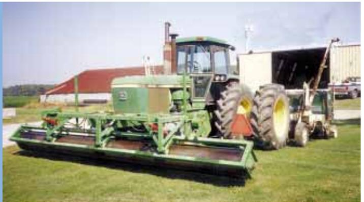
Roberts pushes roller ahead of his Deere 4840 tractor as he plants wheat or soybeans with his 20-ft. grain drill. A pair of hydraulic cylinders are used to tilt roller down.
