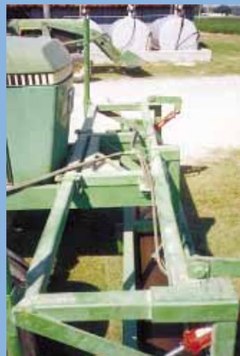
The 18-in. dia. roller mounts on a steel frame that bolts to sides of tractor. The job takes five minutes or less.”
