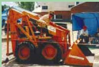
New lift system allows skid steer loader to be used in tight quarters when bucket is down. Counterweight swings in against back of machine.
