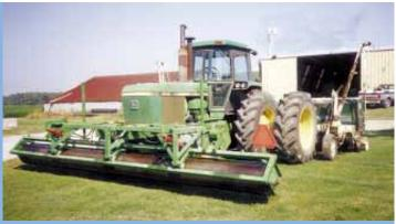
Roberts pushes roller ahead of his Deere 4840 tractor as he plants wheat or soybeans with his 20-ft. grain drill. A pair of hydraulic cylinders are used to tilt roller down.
