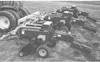
Last winter, FARM SHOW featured my husband Larry's and son Kyle's shop-built splitter hitch that allowed them to pull two Case-IH balers at a time behind a single tractor (Vol. 20, No. 6). The hitch also serves as the hydraulic reservoir for the pumps and 50 hp motors that drive the balers. The hitch worked so well last season on more than 100,000 3 by 3-ft. by 14-in. bales, the men decided the only possible way to improve it was to add a third baler.
