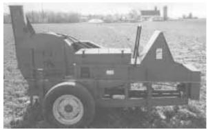
Pto-driven silo blower is equipped with two 9 1/2-in. dia. rollers that crack kernels to boost nutritional value of feed.
