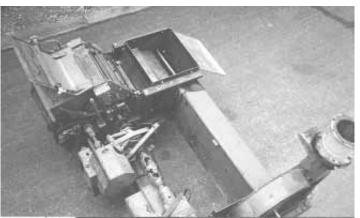
The company also sells a kit for installing a roller mill on a pull-type silage harvester. The blower is moved back 14 in. in order to make room for the rollers, which mount right behind the cutter knives. They recommend removing half the knives in order to offset the increased horsepower requirement. Harvester is shown here with header removed.
