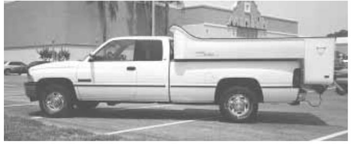
**Lightweight fiberglass box rolls in and out of pickup easily using a winch and lift frame.**
