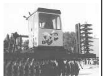
my self-propelled disk can cut it up better and work the soil 10 in. deep. Pitch of the discs, which is adjusted hydraulically, controls the depth at which the discs operate.
