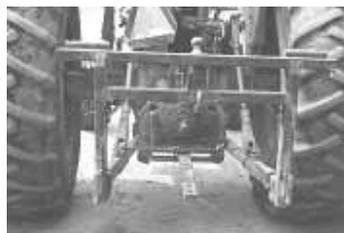
It consists of two 3-ft. uprights 50 in. apart and two crossmembers built of heavy-duty 2 by 4-in. tubing. The top crossmember is fitted with a detachable 2-in. dia. ball hitch, while the bottom crossmember secures to the 3-pt's top link. You can use the hitch to hook up to all 3-pt. mounted equipment, 5th wheel gooseneck trailers, or ball hitch trailers.
