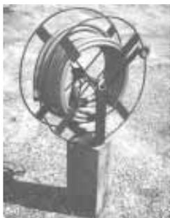
"I used flat stock and steel rods to make a high capacity air hose reel for 1/2 in. dia. or larger hoses. The reel mounts on a swivel made from stainless steel components and turns by grabbing a knob mounted on a handle. I sell them for \$90 without the hose."
