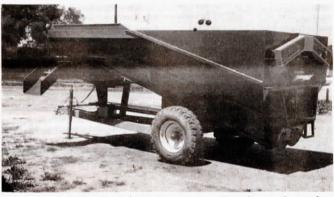
Four augers inside the "slanted" mixer combine livestock, poultry rations at rate of only 2 min. per load.
