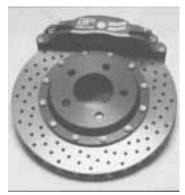
Drilling holes in rotors makes brakes last up to twice as long and improves perfor-
