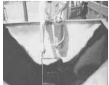
**Spray-on sealant is used to cover spreader at end of season, then reapplied at the beginning of the next season.**
