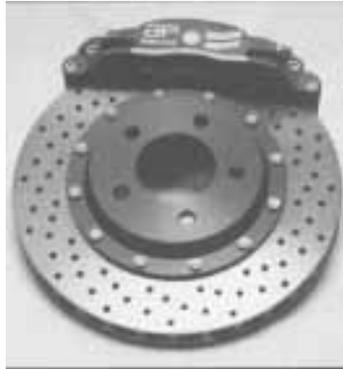
**Drilling holes in rotors makes brakes last up to twice as long and improves performance.**
